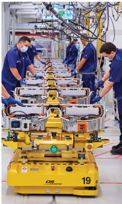
Assembly of incumbent-tech high-voltage battery packs at the BMW plant in Dingolfing, Germany.
