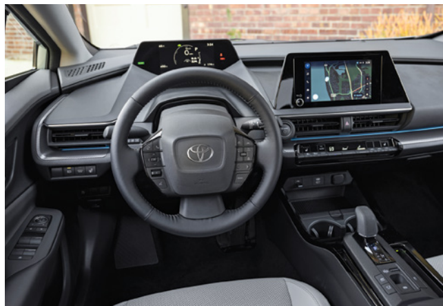
The Prius cabin is completely redesigned to include an instrument cluster directly in front of the driver and the gear selector in a more conventional location.
