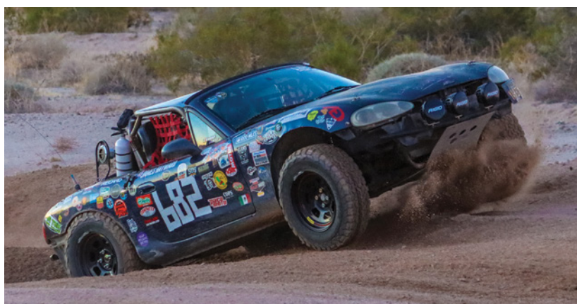
Buddy takes on the two-day Rage at the River desert race in Laughlin, NV before the Perry Parts bump stops were installed. After 60 miles of racing, the passenger front upper shock mount gave up the ghost and we couldn't race Day Two.
