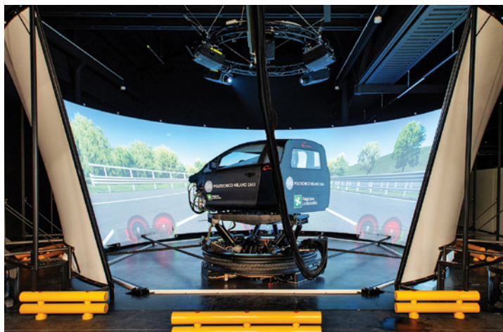
The Politecnico di Milano University used VI-grade’s DiM400 and VI-WorldSim software to improve its test vehicle’s autonomous perception capabilities.
