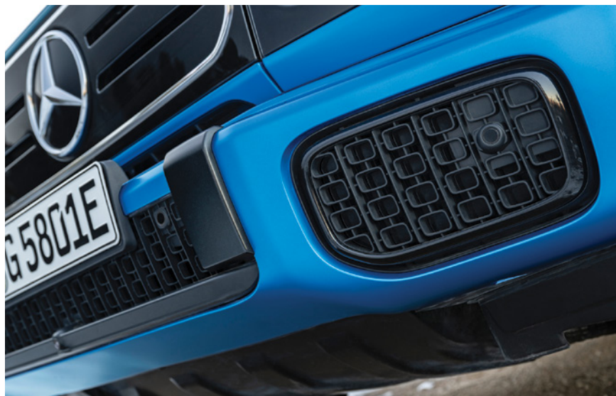
Cameras abound on the new G 580, allowing for a video effect called "transparent hood."
