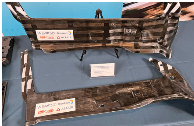
Future of Lightweighting: WEAV3D, Braskem and Clemson Composites Center developed a composite lattice-reinforced polypropylene sheet that reduces cost by 50% and weight by 23% compared to CFPA6 organosheet.
