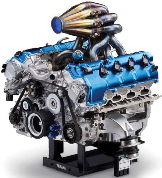
Toyota and Yamaha collaborated on a hydrogen-fueled variant of Toyota's 5.0L V8, which point the way for further hydrogen combustion-engine projects.
