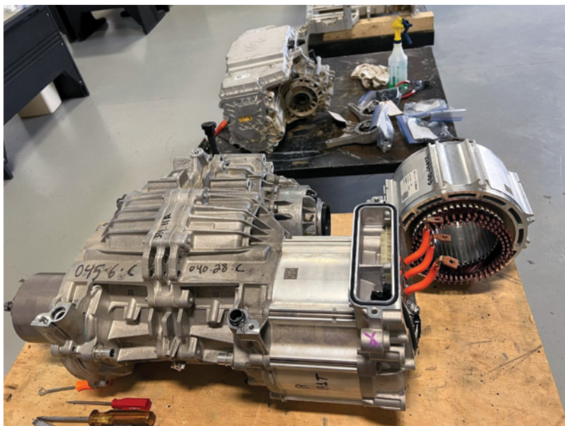
The robust Bosch e-drive units feature hairpin-type motor windings. The motor does not have a heat exchanger/oil pump — it is directly cooled via coolant circulating through channels in the stator housing.
