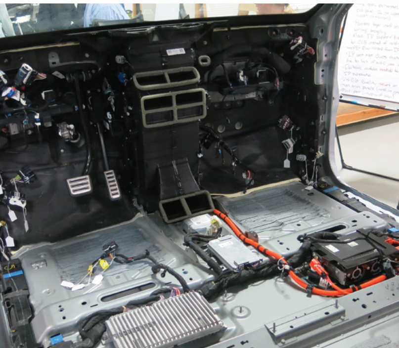
A nearly stripped R1T cabin reveals electronic controller locations, NVH mastics on the floorpan and the innovative HFH cross-car beam.
