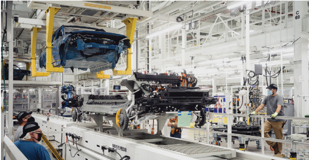
The increasingly common “skateboard” architectures of EVs create unique NVH challenges; here, the chassis of a Rivian R1T pickup is married to the bodyshell at Rivian’s assembly plant in Normal, Illinois.
