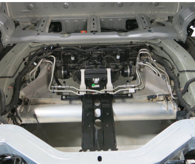
With its composite cargo floor removed, the R1T's rear gearbox, air-suspension components and mixed-materials construction are visible.
