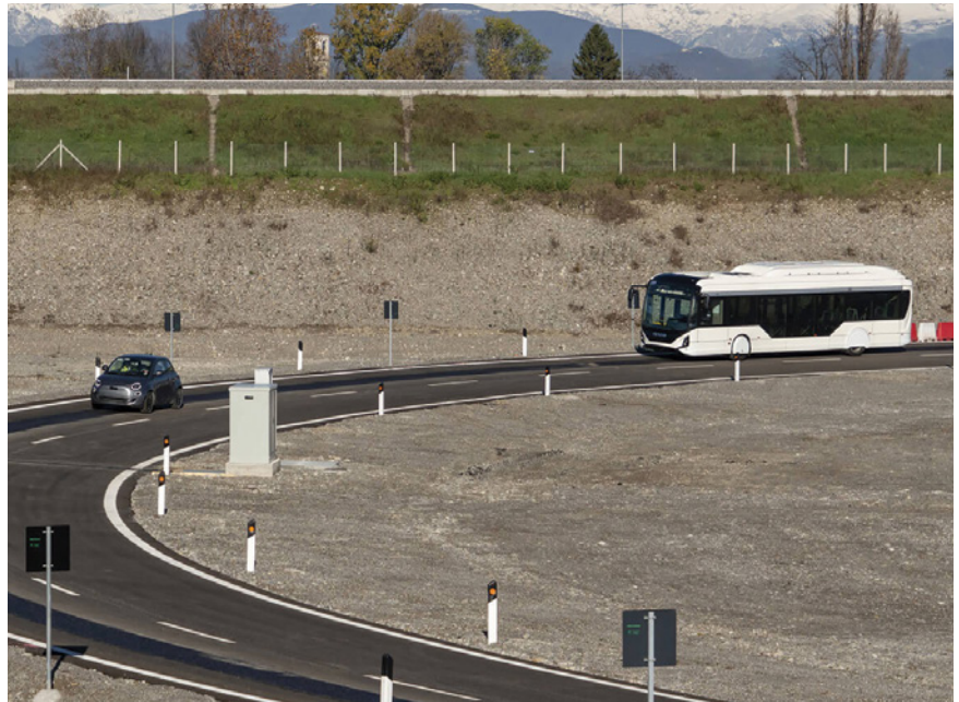
Electreon has integrated its technology at the “Arena of the future” project in Brescia, Italy. Shown are an Iveco electric bus and a Fiat 500-e being charged while driving.
