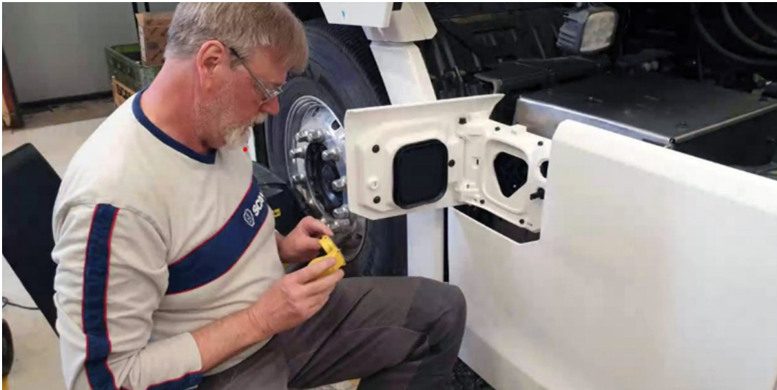
SAE J3271 MCS inlet, similar in size to CCS inlet with 10x (3000 A) charging capability.
