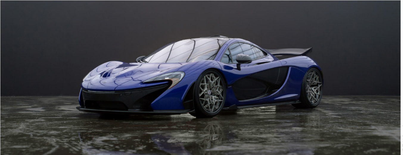
EBM 3D printed titanium wheels.
