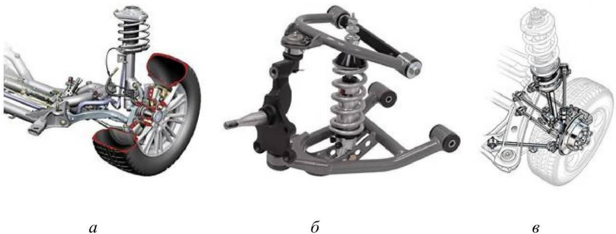
Figure 1 – Types of independent vehicle suspensions: a – MacPherson suspension; b – double wishbone suspension; c – multi-link suspension
